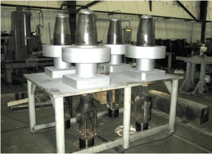
CV's assembled and coated with high temperature paint on non-steampath surfaces.
