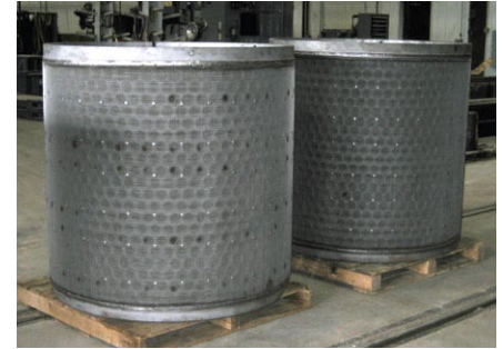
Intercept valve coarse-mesh screens replaced and ready-to-ship.
